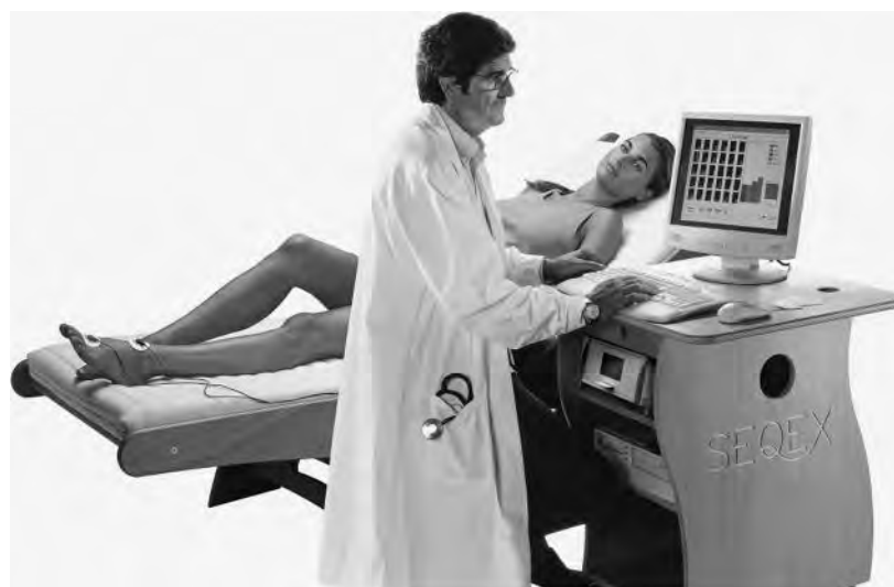
FIGURE 34.20 The Seqex magnetic therapy device (Pergine Valsugana, Italy). One signal shape is selected from an array of 30 wave shapes, the choice depending on the whole-body impedance of the patient. This low frequency signal is repetitively applied by means of coils within specially designed pads that treat the entire body.
