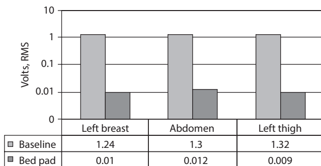
FIGURE 38.8 Effect of grounding with bed pad on 60 Hz induced body voltage. (From Applewhite R Euro Biol Bioelectromagn 2005;1:23–40.)
