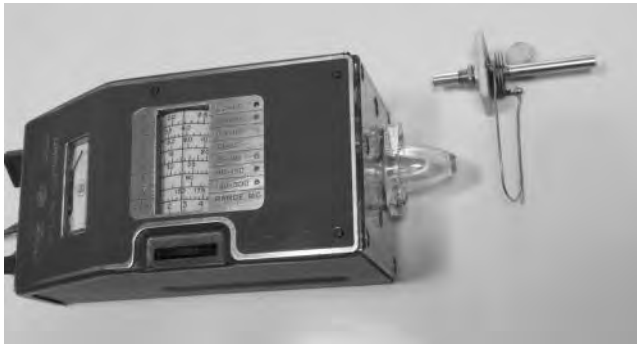
FIGURE 30.5 The grid-dip meter and the passive L/C oscillator simulating an investigated biologic tissue.
