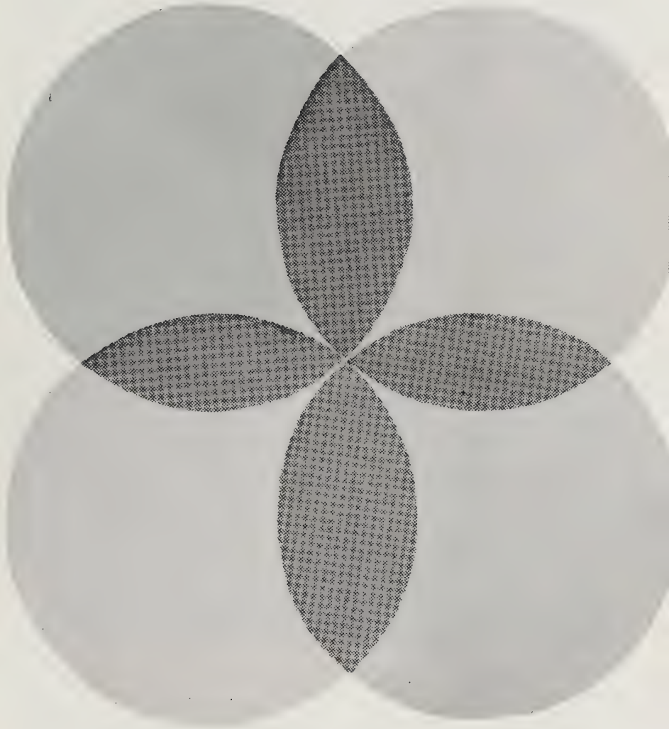
19. An example of Moiré (pronounced “mwa-ray”) patterns, produced when one regular pattern is laid over another. This illustrates the theory that the “Honeycomb” visible in the SPIT-processed photograph may be the product of an actual cellular structure on the landscape, viewed through the “fine mesh” effect produced by the SPIT image-enhancement process.
