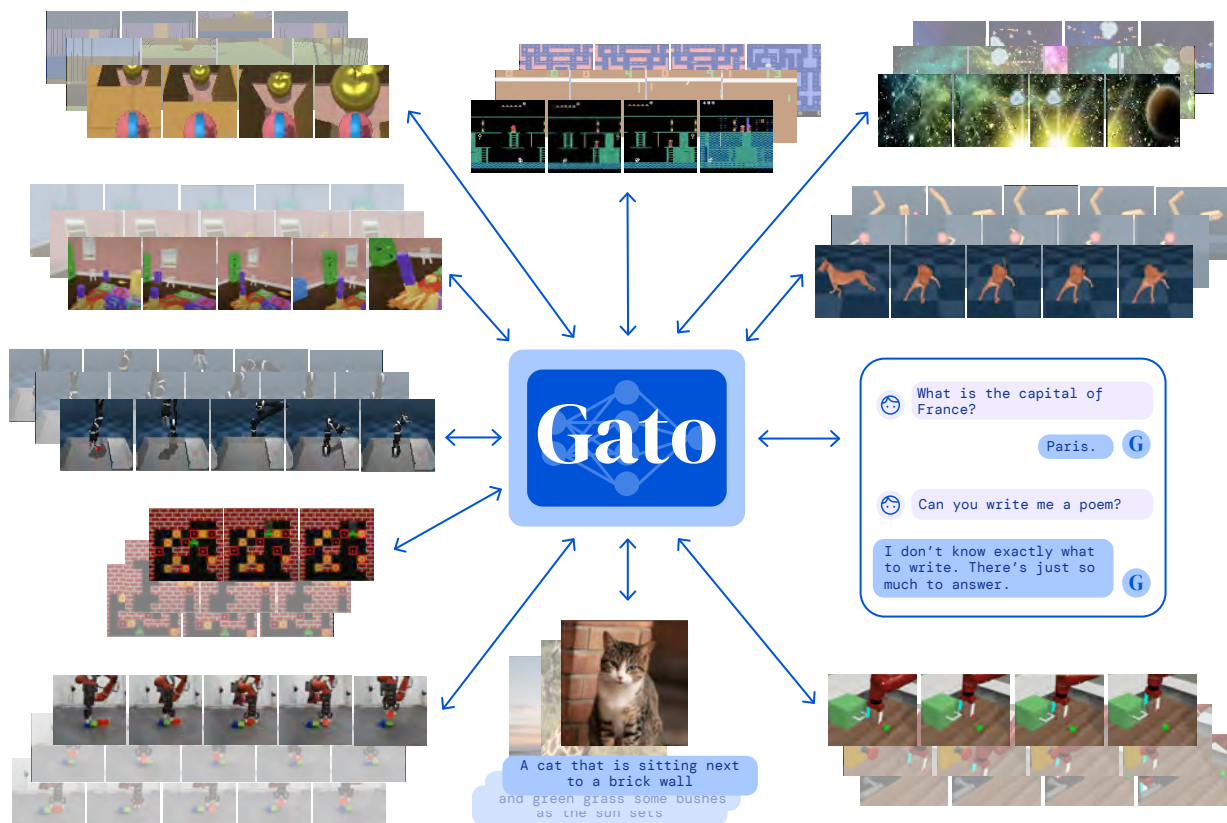
Figure 1 | A generalist agent. Gato can sense and act with different embodiments across a wide range of environments using a single neural network with the same set of weights. Gato was trained on 604 distinct tasks with varying modalities, observations and action specifications.
